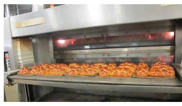
Freshly baked loaves of challah bread leave the three-deck tunnel oven, then are racked and cooled before packaging.
